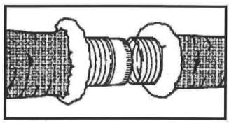
1. Peel back jacket and insulation from core. Butt two cores together on a standard 4"(100mm) metal sleeve.
