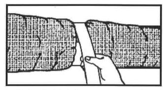
3. Pull jacket and insulation back over cores. Tape jackets together with at least 2 wraps of duct tape. A clamp may be used in place of or in combination with the duct tape.
