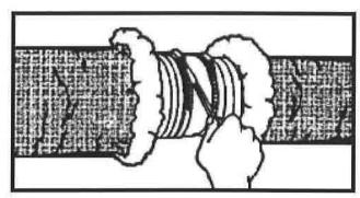
2. Tape cores together with at least 2 wraps of duct tape. Secure with 2 clamps.
